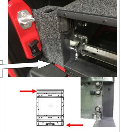
2.08/- Fit left "L" support brackets to the left corner of the drawer assembly. Fasten with 3X M6 hex head bolts from inside the drawer assembly. Ensure slots for floor cleats face the rear of the vehicle.
