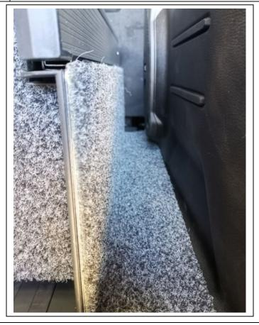
2.10/- Fasten the panel marked CECC JLSUB using the (4) 6mm x 20mm black round head set screws to the exterior of drawer on side that has subwoofer mounted to vehicle. This panel will provide a carpet finish to the exterior of the installed drawer.
